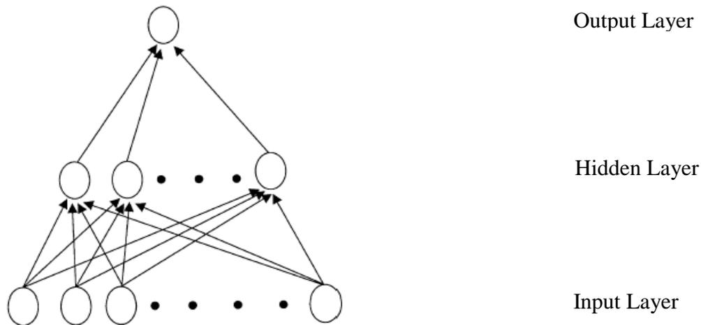
**Figure 1. Architecture of multilayer feed forward neural network.**
